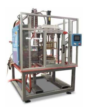
The Radyne Braze-Press™ is a turn-key controlled atmosphere brazing system ideal for applications that require oxidation-free braze joints without the use of flux.
