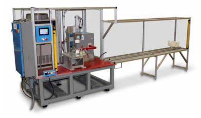
The Fluid & Fuel Line brazing system from Radyne offers an ideal solution to brazing joints, brackets, and fittings on long runs of tube. This system features nitrogen or argon controlled atmosphere chambers for clean, oxidation-free braze joints without the use of flux. Removing toxic and costly flux from your processes can help keep your production facility clean and safe.
