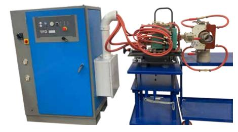
The Radyne Large Tube Brazing Workstation is designed for some of the largest and most demanding brazing applications. The system features a compact heat station mounted to a movable and height adjustable cart. Our specially designed inductor features quick disconnects for the outside half of the inductor and water lines. This allows for long, complex tube runs to be brazed with ease. The inductor and heat station can also be rotated 90 degrees for horizontal, vertical, and angled brazing.
