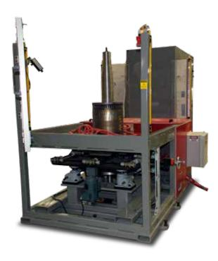
The Radyne Rotor Brazing System is designed for brazing copper ring end caps to large rotor assemblies for electric motors. Our uniquely shaped inductor is designed to evenly heat the round and flat surface of the ring for a consistent braze joint all the way around. This machine can also be easily adapted to braze other large, round, and flat objects.
