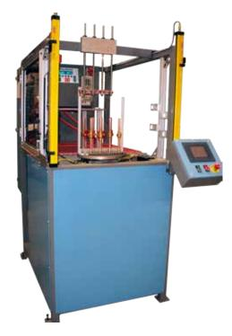
The Radyne Lift and Rotate Brazing System is an ideal way to increase production rates while retaining a compact footprint. The rotating part loader assembly allows a single operator to stage the next batch of parts while the heat cycle is occurring. This reduces operator and machine idle time and increases production rates. The part loader can be customized to fit unique part shapes and sizes. This system is also easily integrated with robotic material handling systems.
