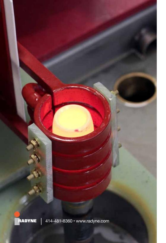
Induction heating is fast- a properly tuned induction heating machine can process high part volumes per minute by utilizing efficient coil design and part handling.
