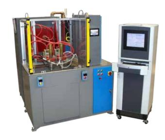
Radyne Large Caliber Ammunition Annealing Systems are designed for the largest ammunition casings on the market today. These systems are able to anneal two 30mm-105mm casings at once and are compatible with brass, steal, and most alloys.
