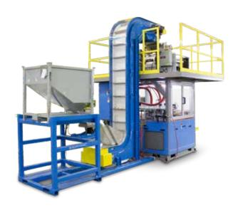
Radyne Cartridge Annealing Systems use a continuously fed indexing system designed to anneal ammunition casings with extreme precision. Integrated quality control systems provide for precise annealing profiles. Cartridge Annealing Systems with single or dual feed streams are available based on your production rate needs.
